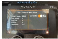
to enable the autostandby mode select the switch in on position: color active,
