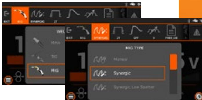
Synergic MIG Welding: Synergic MIG welding is an advanced version of MIG welding that incorporates technology to simplify the welding process. This type of welding uses a synergic power source that automatically adjusts the welding parameters based on the selected wire feed speed. The technology ensures that the voltage and current settings are optimized for the specific wire feed speed, reducing the need for manual adjustments.
